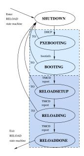
Figure 1: The Emulab node-imaging state machine.
