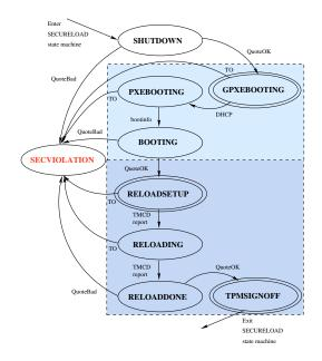
Figure 2: The Emulab TDLS state machine.
