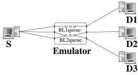
Figure 4: An abstracted view of Figure 3, with the bottleneck links represented as bottleneck queues.
