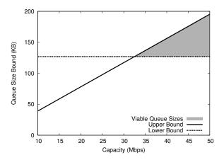
Figure 1: The relationship between capacity and the bounds on queue size for a path with  $ABW_f = ABW_r = 10 \text{ Mbps}$ ,  $RTT_{base} = 20 \text{ ms}$ , and  $w_{max} = 65 \text{ KB}$ . Low capacities prevent any viable queue size.
