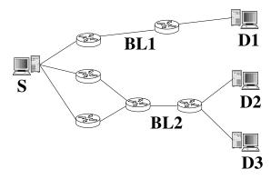
Figure 3: A router-level topology, showing two bottleneck links. One (BL2) is shared by two paths from source S: the paths to destinations D2 and D3.
