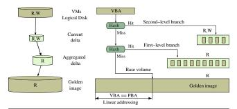
**Figure 3.** Three-level branching storage with a corresponding virtual block address translation scheme
