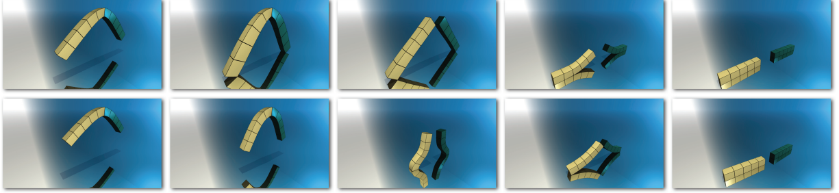
Figure 8: Top row: Animation sequence of an elongated bar undergoing deformations based on the infinitesimal strain tensor. The lack of nonlinear terms causes large distortions and ghost forces in the shape. Bottom row: By filtering high frequencies from the forces based on the finite strain tensor, a larger timestep and nonlinear deformation behavior can be achieved.
