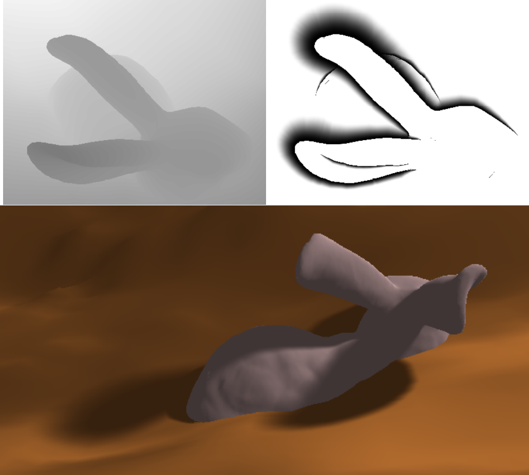
Figure 3: An example shadow map (top left), corresponding penumbra map (top right), and the final rendered result.
