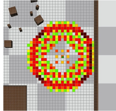
Figure 3: A snapshot of 2D-TLM sound propagation model. P is a sound packet in one grid.
