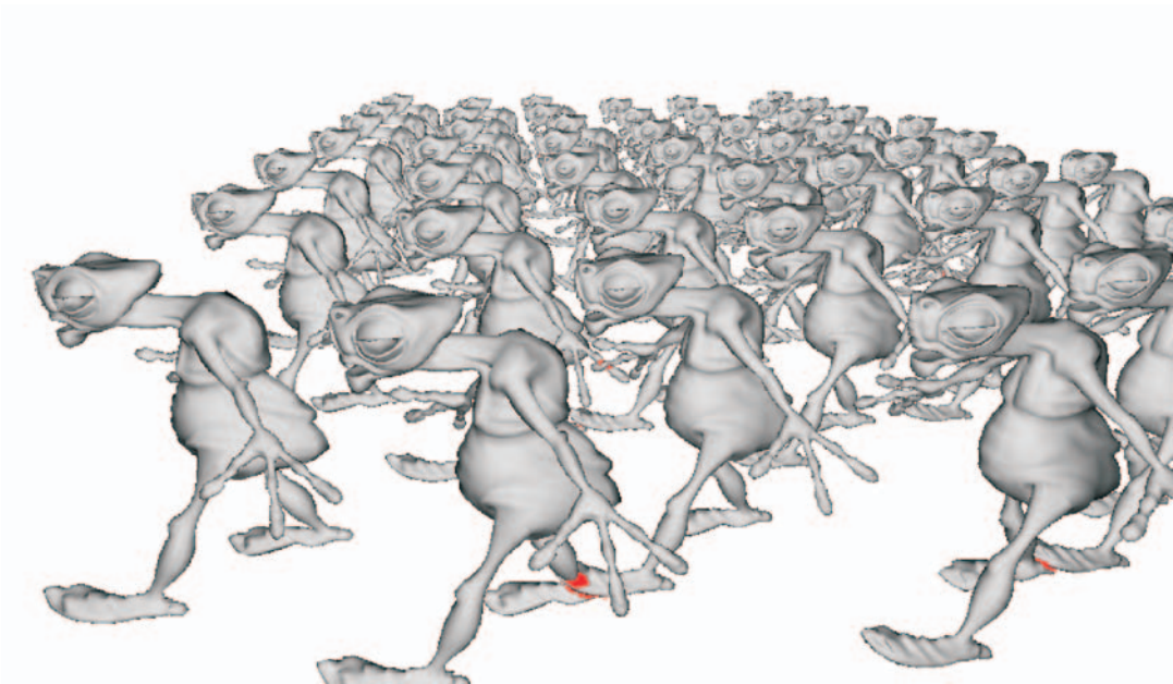
Figure 5.7: The scenario for our crowd collision detection experiment: 50 animated creatures with more than 650 thousands triangles together. Our CD algorithm needs an average 52.83ms per frame, whereas the CD based on complete BVH refitting takes 779.3ms (15-times more).
