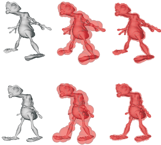
Figure 4: Top: reference posture of the creature with spheres on levels 4 and 6 of the tree (precomputed according to section 3.1), down: an animated posture with spheres refitted by our algorithm (during run-time).
