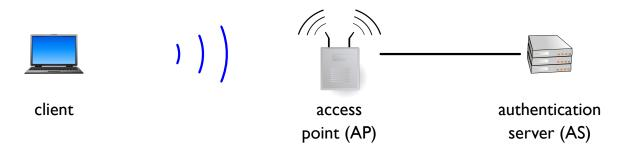
Supports an **authentication server (AS)** that is separate from the Wi-Fi **access point (AP)**
