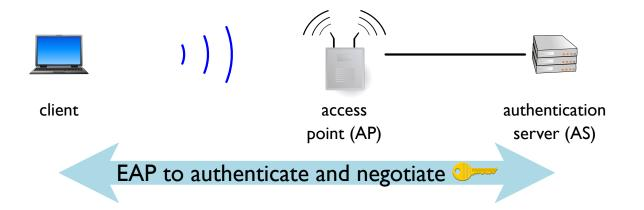
The AP then acts as a bridge for client and AS to pick a master key using the **Extensible Authentication Protocol (EAP)**
