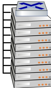
Top of rack (TOR) switch
